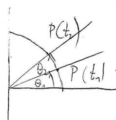
$$\bar{\omega} = \frac{\theta_2 - \theta_1}{t_2 - t_1} = \frac{\Delta \theta}{\Delta t} \quad [\frac{1}{s}] \quad \left\{ \begin{array}{l} \text{dla danaego prędkości} \\ \text{wykonanie kąta} \end{array} \right.$$
